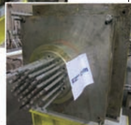
Fig. 2-2 OVM250-43 cable anchor head (fixed)
